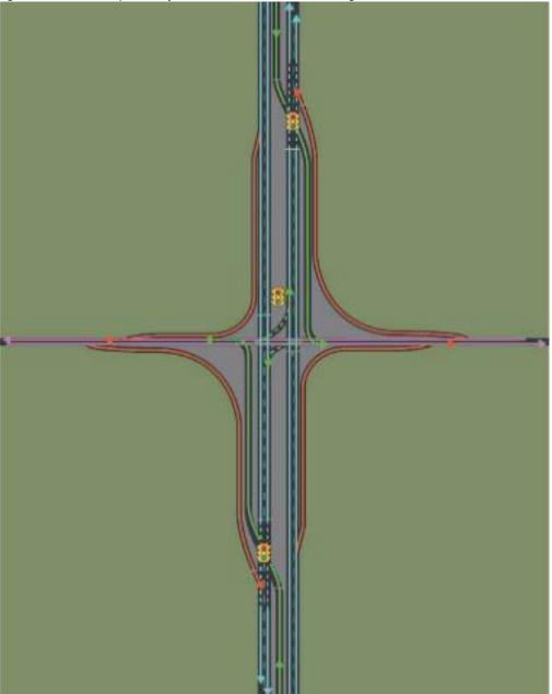
Figure 2-14: Partial Displaced Left Turn Intersection Schematic Diagram
