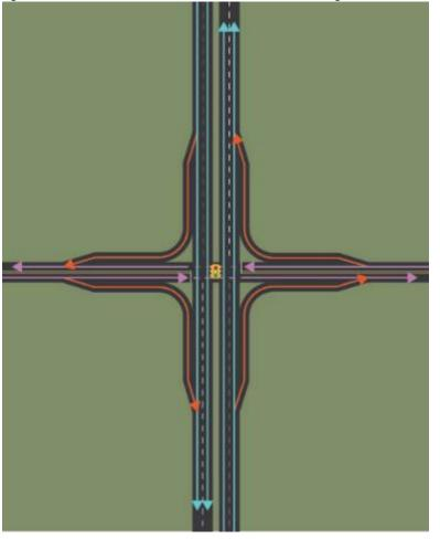
Figure 2 4: Acceleration and Deceleration Lanes Schematic Diagram
