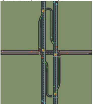
Figure 2-11: Boulevard Left Turn Schematic Diagram
