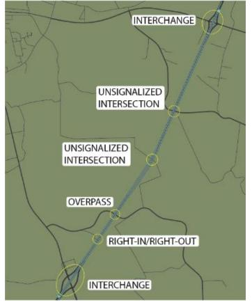
Figure 2-3: Free Flow Facility Example with Partial Access Control
